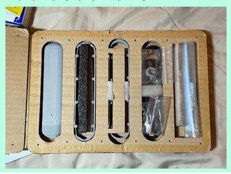
Front left to right, are the (1) roof, the (2) window areas, the (3) lower left side and ends, the (4) parts bin including the side frames, detail parts and the special part 1255B for the Bowser 125115 traction drive and the (5) window glasses. Also a very detailed instruction sheet showing assembly and painting instructions is provided.
